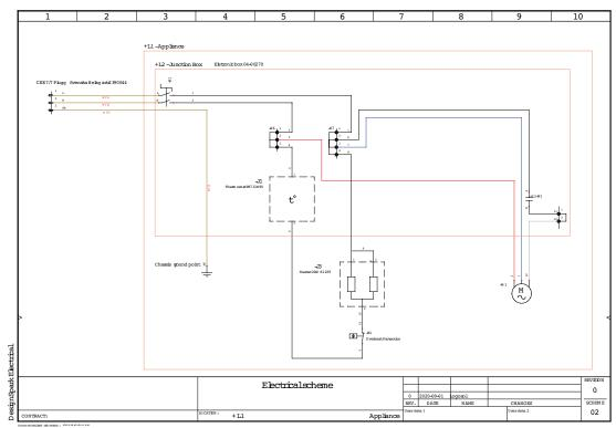
Wiring diagram is found inside the junction box of the drying unit.
