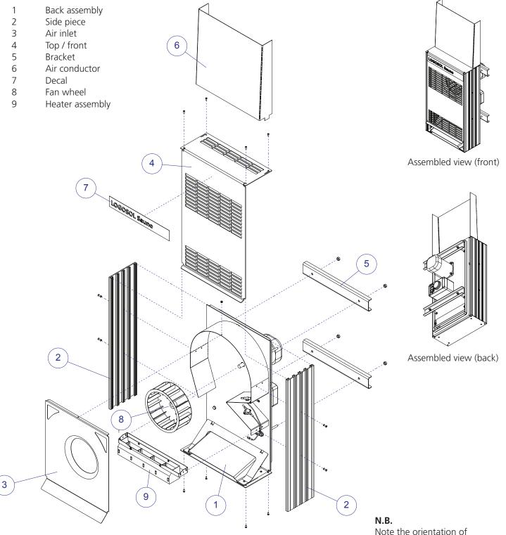
Note the orientation of pos. 2 (the longest distance between hole and edge should be facing upwards).
