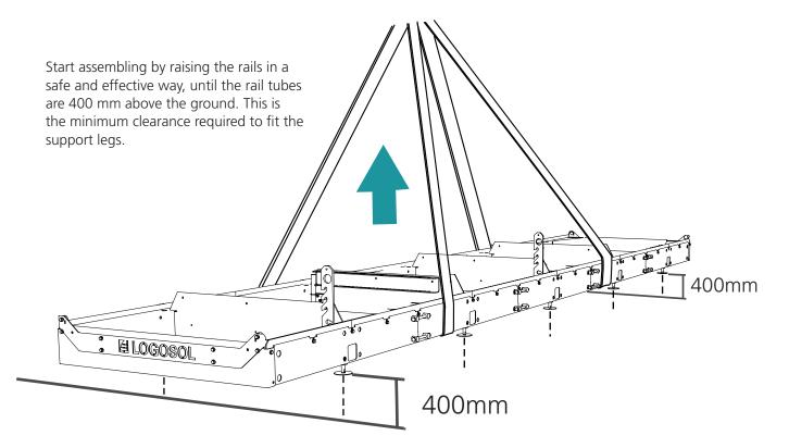
Recommended positions of the support legs on the rail frame.
